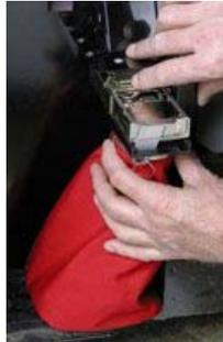
Release the latch on the machine mounted universal funnel assembly that hold the coin bag with the patented locking mechanism.
