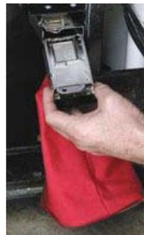
Reinsert an empty coin bag into universal funnel assembly. Locking mechanism on bag will automatically open and latch into place.
